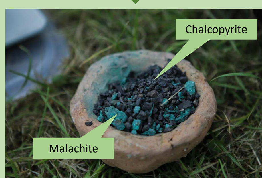
The roasted ore was crushed, placed in a crucible and mixed with sand and charcoal. In three of the experiments the chalcopyrite was mixed with another ore: malachite.
