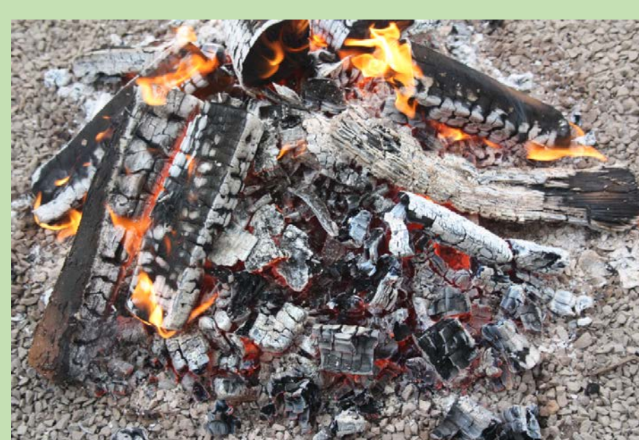
Chalcopyrite ore was roasted in a fire at approx. 800°C for 12 hours.
