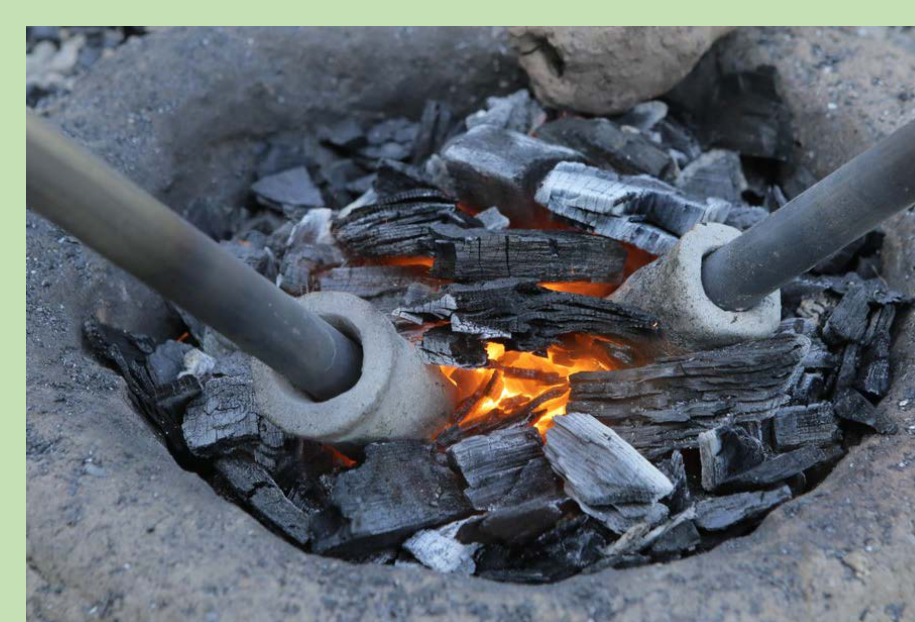
A fire was lit within the bowl shaped furnace, and the crucible placed in the centre. The crucible was completely covered with charcoal in order to exclude oxygen.
